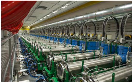
← AIRIX machine -Accelerator cells
